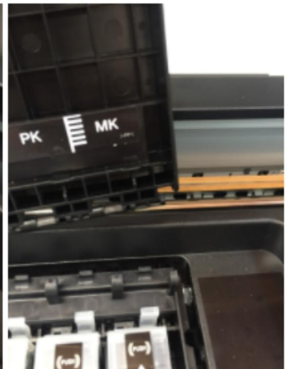
**Ink Cover Switch:** There is a small switch provided with your ink set or cartridge. It tricks the printer into thinking your ink cover is still down (even though it's not even there). After installing the cartridges, place this switch into the correct slot as shown below. Note: Always take the switch OUT before doing anything with cartridges. Put the switch back after inserting your cartridge(s).
