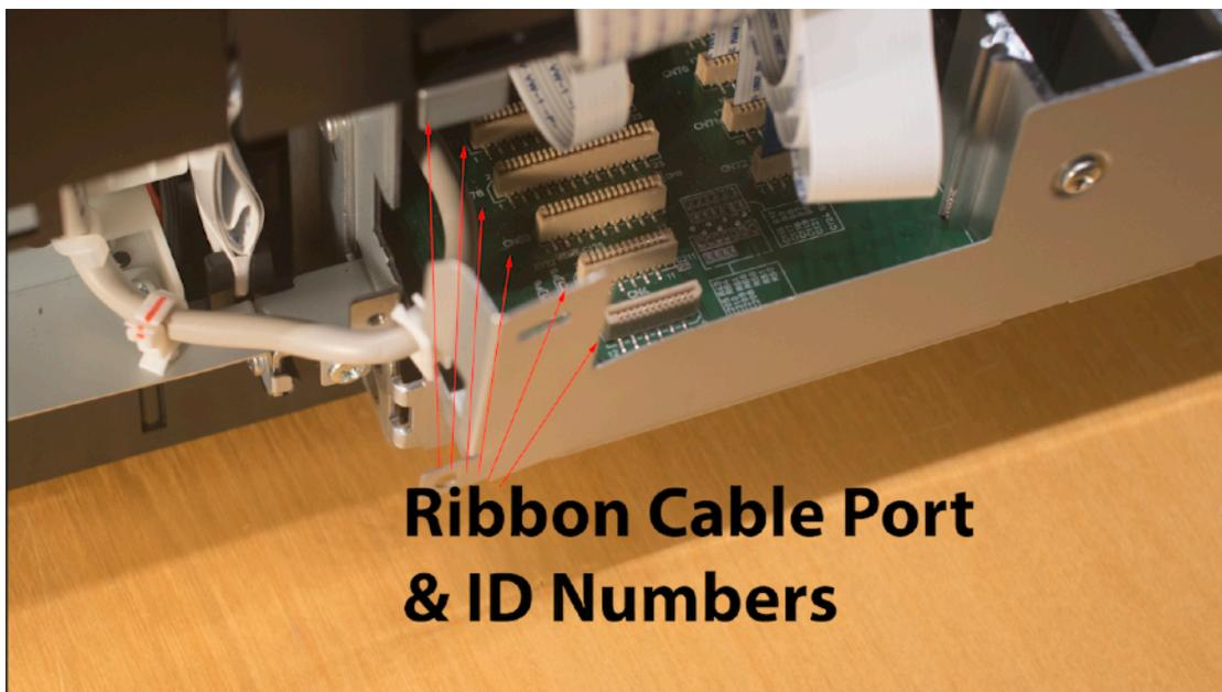
10. These cables can be very tricky to place correctly. Do not touch the metal contacts. Carefully guide the cable to the lip of the port and then gently push in. The cable can be bent slightly (at a 90 degree angle) to give you fingers leverage to push the metal contacts all the way in. They will make a dull “thud” and level off when they are all the way in. Do not fray the cable.
