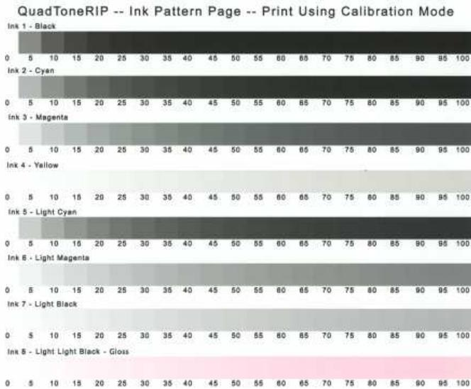
Illustration 9 QuadTone RIP Calibration Mode printout from an Epson 7880 Piezography K7 system
