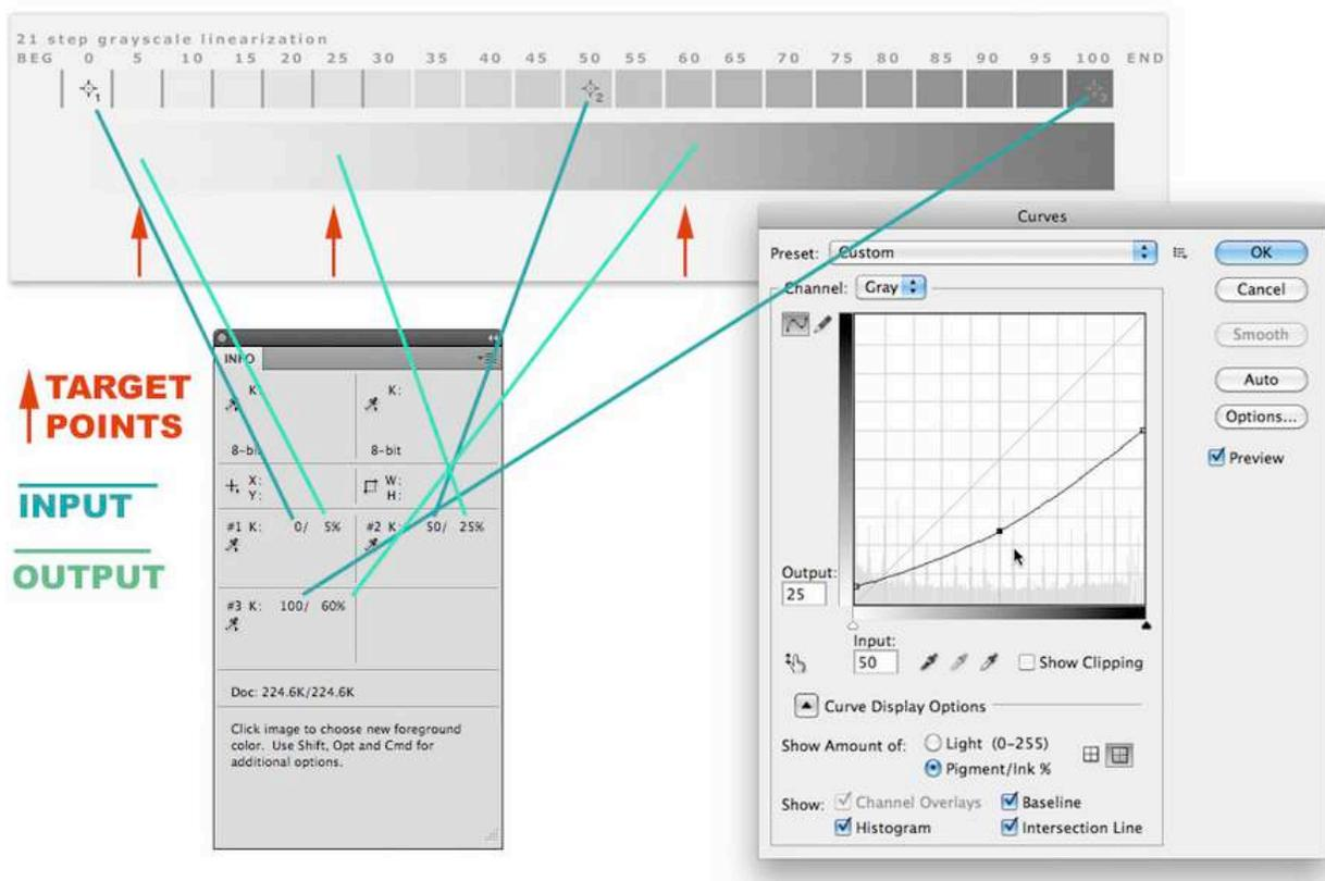
This is the curve that you might use on your inverted digital images before printing them to the Piezography digital film system were your process to imitate this example. But, it is only an example of a curve and it does not mean you do not have to go through the process yourself!
