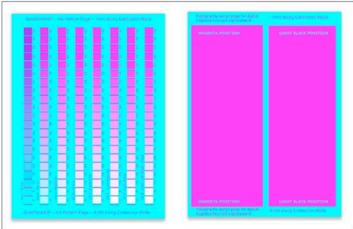
Above on the left is the regular QTR Calibration Mode image. It is a color image that uses specific RGB values to trigger each ink shade to print when using the QTR RIP. Calibration Mode is a special QTR mode that is used when attempting to make your own QTR curves using the QTR Curves Tool. We will use this special mode to purge your printer using a special purge target that is made of two of the patches on the regular QTR Calibration Mode target.
