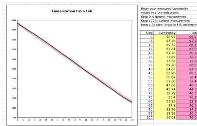
Illustration 7. Linearization displayed by pasting L values from spreadsheet on illustration 6.
