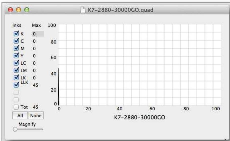
Here is a typical GO Curve. There is only one ink position printing and it does not actually appear to be very curve like. It is actually a single digit encoded into the entire curve. GO is installed in the LLK position. And the value that is normally always kept at 0 for every member of a curve has been changed to 30,000. That value is recorded in the L255 slot of the LLK curve. 255 is
