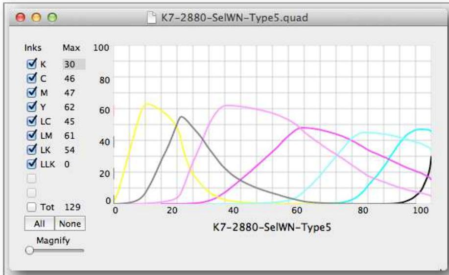
This is a Piezography Glossy inks curve that was custom made for a customer using a split tone ink set of Selenium and Warm Neutral inks. The Selenium inks are in the shades 7 through 5 represented on this curve view by the color slot location in the printer (yellow, light black, light magenta). The Warm Neutral inks are in shades 4 -1 represented on this curve view by the color slot location in the printer (magenta, light cyan, cyan and black).
