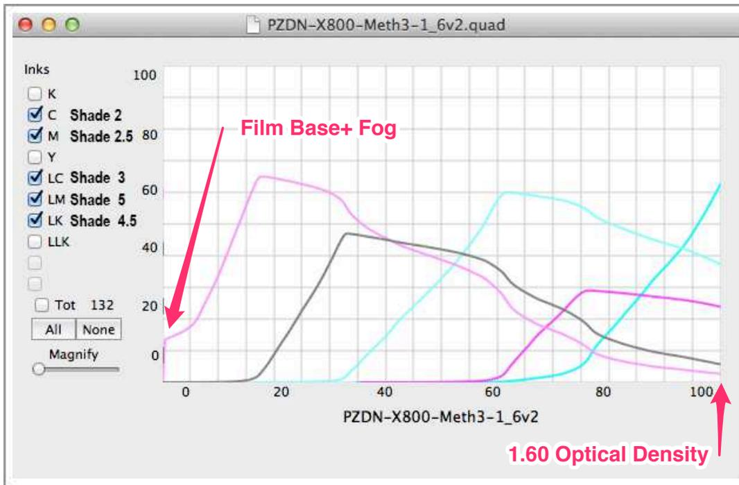
The Piezography Digital Film 1.60 QTR curve for typical silver fiber based paper or RC paper.
