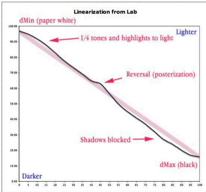
Illustration 8 – Examples of poor linearization problems.
