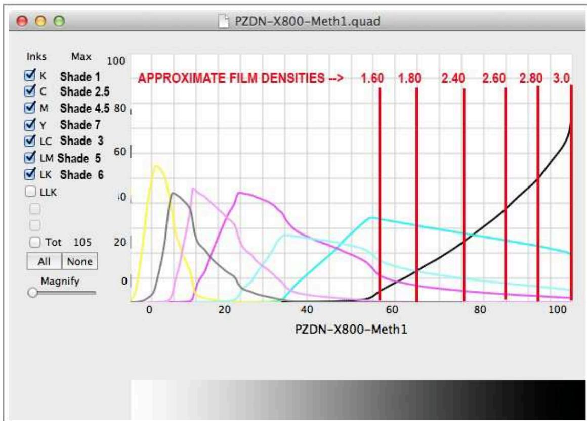
The actual QuadTone RIP curve "PZDN-X800-Meth1". This process uses Piezography MPS Selenium black shade 1, Selenium shades 2.5, 3, 4.5, 5, 6, 7. You will need to limit your output density in Photoshop according to the dMax required by your alternative process or silver paper. By limiting your output you can fit the image file to the density you require. If the black point of a Photoshop image were reduced from 100% to about 60%, it would produce a film optical density of about 1.65.
