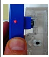
Left: Close-up of the chip resetter in contact with a cartridge chip. Note how the gold contact pins are centered over the green chip, so that each pin contacts a rectangular pad on the chip.
